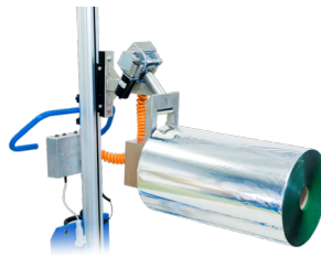
Expand&Turn - pneumatic expander, turning operated electrically
